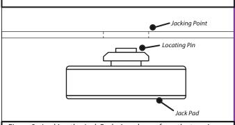
Figure 3 - Locking the Jack Pad, view shown from the top view. The twist results in the pin sitting on the topside of the jacking point
